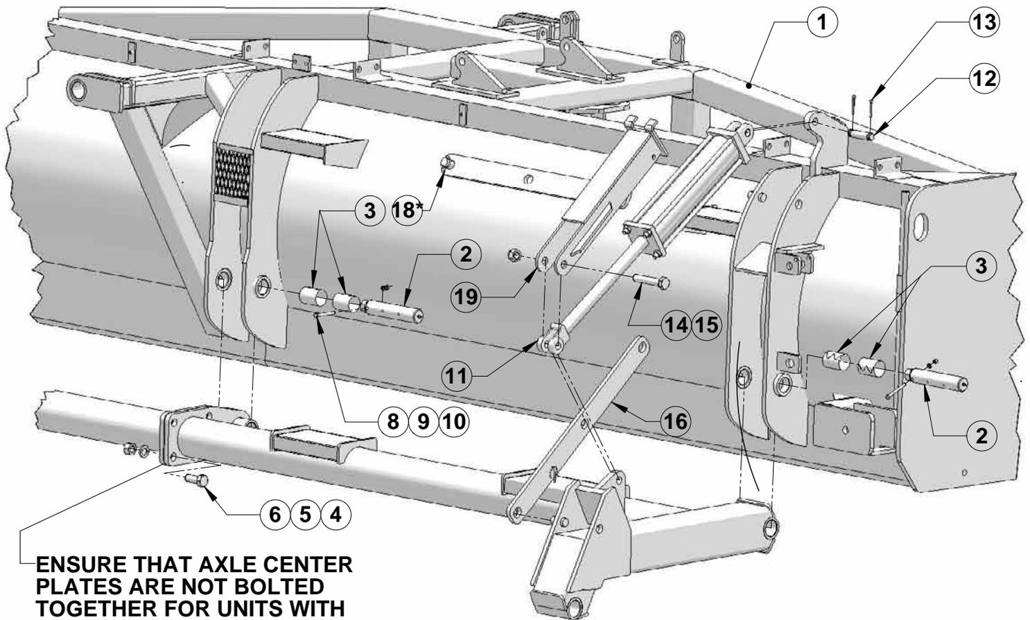
**ENSURE THAT AXLE CENTER PLATES ARE NOT BOLTED TOGETHER FOR UNITS WITH TWO TOWERS!**
